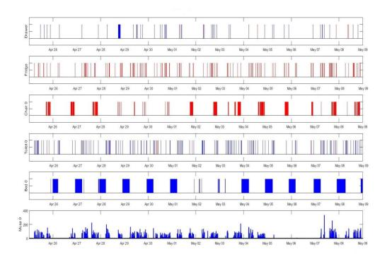
Figure 3.1: some raw data from NL\_02. The six plots represent, from top to bottom, Drawer, Fridge, Chair, Toilet, Bed and MuSA. A red or blue line signals the device activity in that moment
